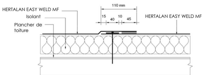
Fig. 8: - Joint longitudinal HERTALAN EASY WELD MF
