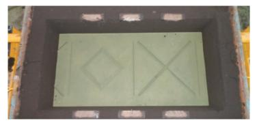
The main difficulty resided in defining the dimensions of the panels taking into consideration the deformation of the metal caused by stamping, and at the same time ensuring the system remains watertight. And subsequently in creating the stamping and bending die to test the quality of the product.
